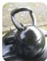
Tilt & pivot handle to adjust flow to 'waste'
